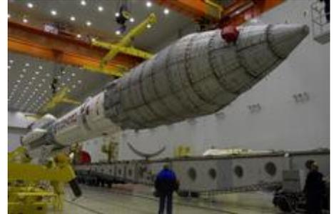
Hardly a vacation spot, this is where the Breeze M low pressure tanks are filled. This is another one of those hazardous operations which required evacuation of the Processing Facilities (including offices).
