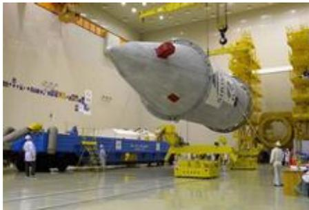
(PLF) halves, which will protect the satellite during its ascent through the atmosphere. The resulting structure, still attached to the tilter, is now known as the Ascent Unit (AU, [See Photo Gallery](#).)
