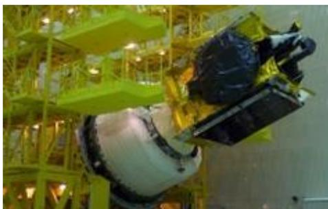
Back on 28 March, we started combined operations, a major milestone in the program. Up to this point, the SC and LV teams had been doing their work in "stand-alone" mode, getting the LV components ready, checking on the health of the SC and finally fueling the SC. Finally, the SC was moved to the mating area, attached to the payload adapter (PLA) and secured via the installation of a separation system ring. This SC/PLA assembly was raised in the tilter stand to and joined with the upper stage of
