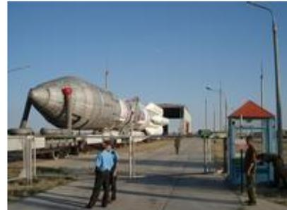
The unit was towed out via a locomotive, and then backed up into the Breeze M fueling station, which looks like a huge carport of sorts. This is its home for two days as the Breeze M multi-burn main engine takes on fuel. All fueling operations are completely controlled by Khrunichev specialists.
