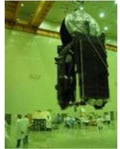
The SC is well protected within the container, so we left it there overnight. Early the next morning, the riggers came in and started the process of removing the SC from its container. This entails removing the lid, rotating the SC from horizontal to vertical, and using the crane to life it off its supports.
