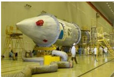
Very little time was wasted before the AU was mated to the launch vehicle (LV). With the AU on its rail dolly, Khrunichev specialists hand cranked the unit and aligned it with the LV. Mating operations were performed and, as we always like to report, there were no anomalies. It is finally one complete unit, known as the Integrated Launch Vehicle (ILV).
