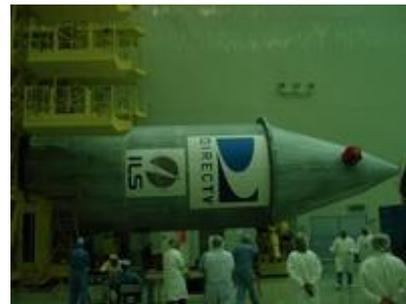
Once the two halves are secured, the team spends two days performing electrical tests and verifying that, although encapsulated, it is still possible to communicate with the SC. The term "team" certainly applies in this case, as a veritable plethora of activities are ongoing while the Boeing folks and the Khrunichev teams work together performing pre-launch testing.
