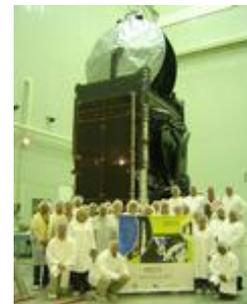
Saturday, the SC-adapter-Breeze M stack will be rotated from vertical to horizontal and the payload fairing installed. The combination of all these pieces into a single unit is known as the ascent unit (AU). The SC will remain in a horizontal orientation until we move the whole launch vehicle to launch pad on L-5 days. This differs from U.S. launch vehicle processing, in that the majority of assembly occurs horizontally. Quite a difference if you are not used to it!
