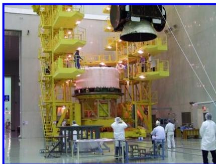
At 6 a.m. bright and early Wednesday, crews reported in to mate the SC to the adapter. The plan was to do the mate, perform electrical checks, lift the SC and adapter, mate it to Breeze M, and follow up with electrical checks again, all in one very long day and night. We actually extended the operation into Thursday, and successfully lifted and mated the SC to the Breeze M. Then the test team came in, and we are on track.
