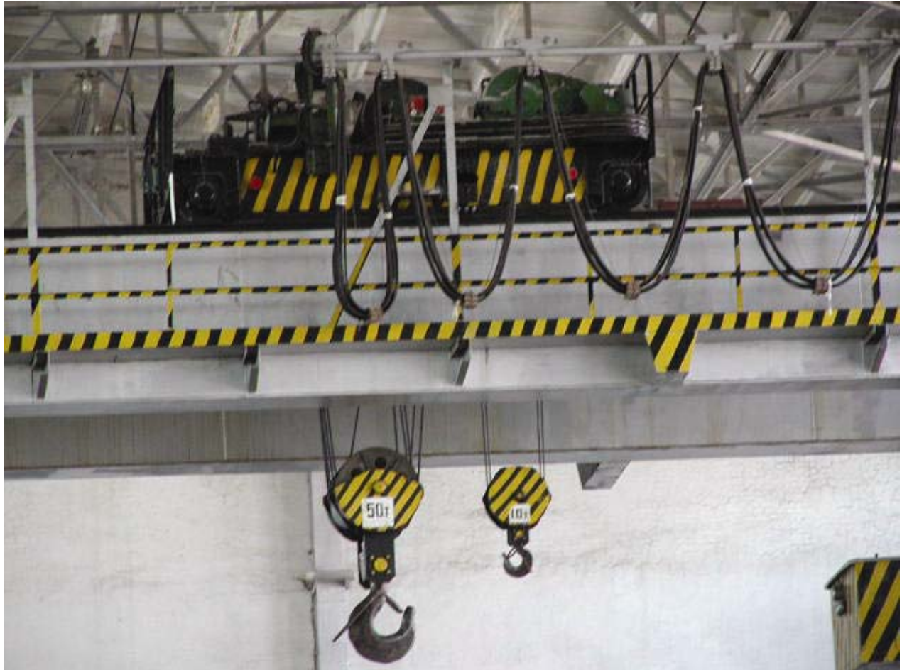
Figure 6.2.2-2: 50-MT and 10-MT Crane Hooks in Hall 102
