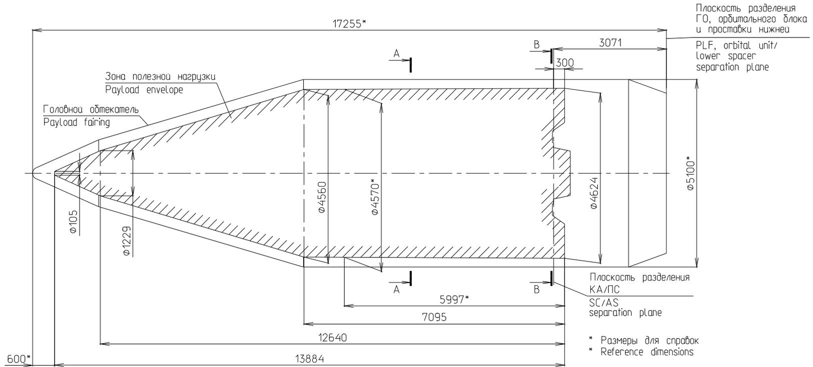
Figure F.7-1b: Payload Envelope Under Proton Breeze M 5-Meter PLF Fairing (Sheet 2 of 2)
