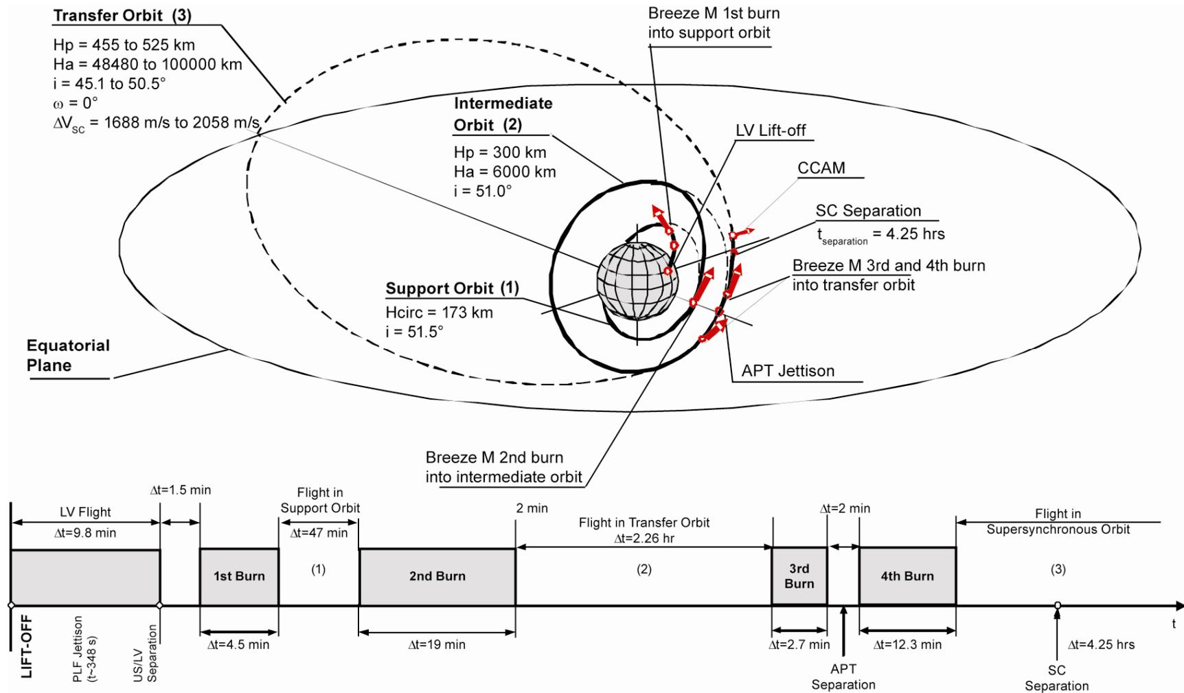
Figure F.4.1-2: Typical Proton M/Breeze M Ground Track for SC Perigee Injection into SSTO ( $H_a = 100,000$  km) Using a 4-hour Timeline from the First Ascending Node of a Parking Orbit Inclined at  $51.5^\circ$
